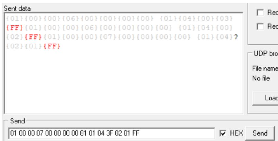
At this point, the camera should have moved to Preset #1, if it was configured.
